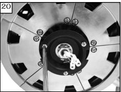
Loosen 2 screws with key slots and remove the 1 screw with closed slot. Save screw removed.
